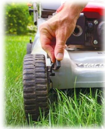
A close-up photograph showing a person's hand adjusting the cutting height of a lawnmower. The hand is pulling a lever on the side of the mower, which is positioned on a lawn with tall grass.
